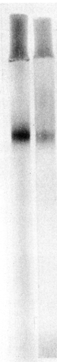
Figure 3. Polyacrylamide disk gel electrophoresis of isolated pea lipoxygenase isoenzyme-1. The sample size was 30 \mu g of protein/gel (7.5% acrylamide, 0.2% bisacrylamide). Gels were stained for protein (left) and activity (right). The current was 2.5 mA/gel for the first 20 min and then 3 mA/gel for 1 h at 4 °C.
